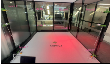
(b) The physical experiment setup showing the Crazyflie 2.1 UAV positioned at the center of a red flight zone.
