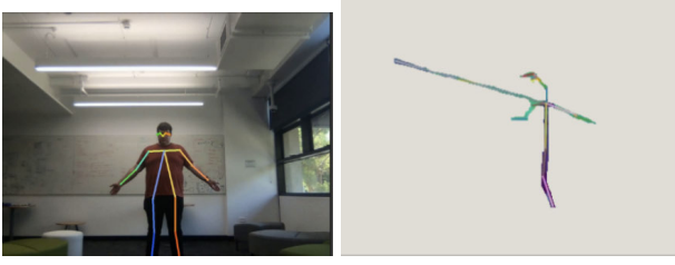
Fig. 2. Observations without using proposed CKD framework. Left: teacher class over original video frame with Alphapose detection. Right: student class CSI-trained model and pose detection using classic knowledge distillation.
