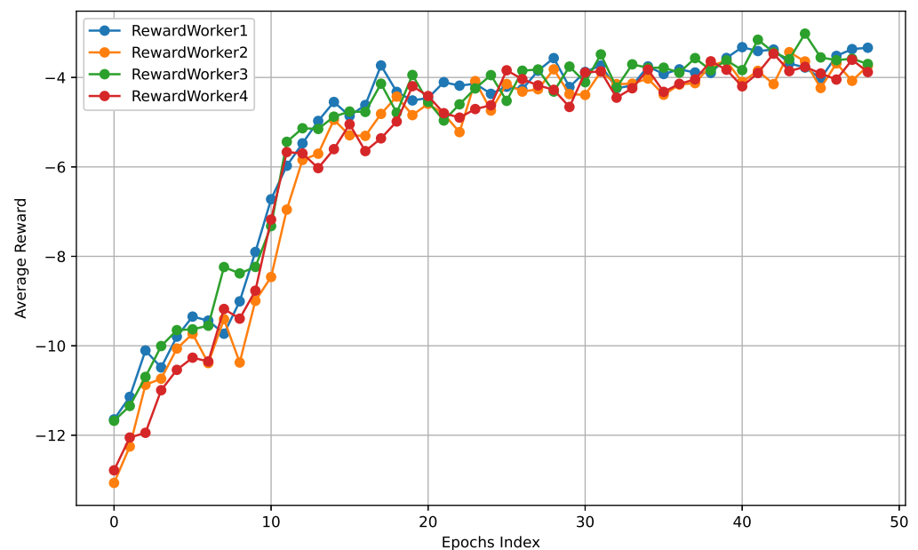
Figure 25. Evolution of the average reward ( R_t ) of the trained A3C model over the entire fifty epochs.
